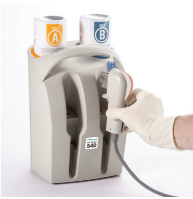
The cable head, with sensor attached, is placed in the calibrator.
